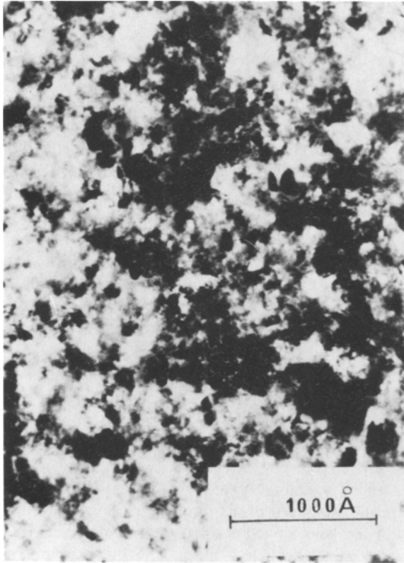
Fig. 4. TEM micrograph of Al-Ge thin mixture film with \sim 30\% vol. Al. "Blacks and whites" do not refer to the different constituents but to different orientations.
